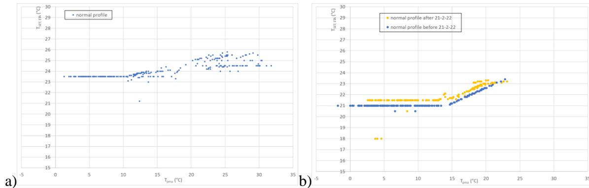
Figure 7: Desired indoor temperature as a function of the prevailing mean ambient temperature  $T_{pma}$  for the house in Italy (a) and in Luxembourg (b). During the course of the year, the residents sometimes change the settings, which - in the case of the house in Luxembourg - has been indicated with blue and yellow dots.
