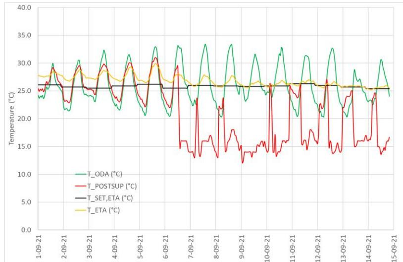
Figure 4: Cooling effect of the system before and after activation of postcooling. Lines indicate temperatures of outdoor air (green), supply air after postcooling (red), extract air (yellow) and setpoint for extract (black).
