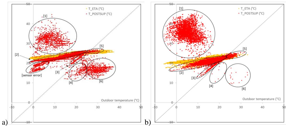
Figure 5: Temperature correlation of supply air (red) and extract air (yellow) as a function of outdoor temperature for the house in Italy (a) and in Luxembourg (b)
