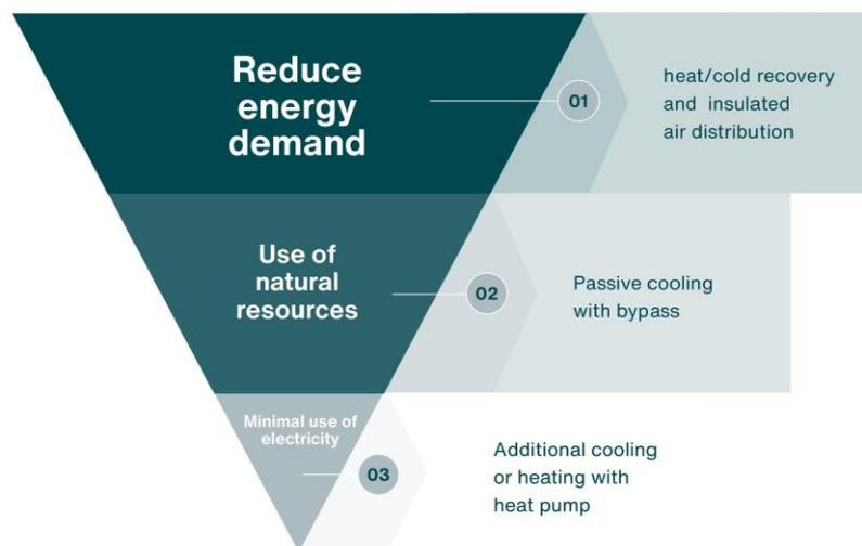
Figure 6: The concept of the Trias Energetica and the implementation for balanced ventilation with postconditioning by an air-to-air heat pump
