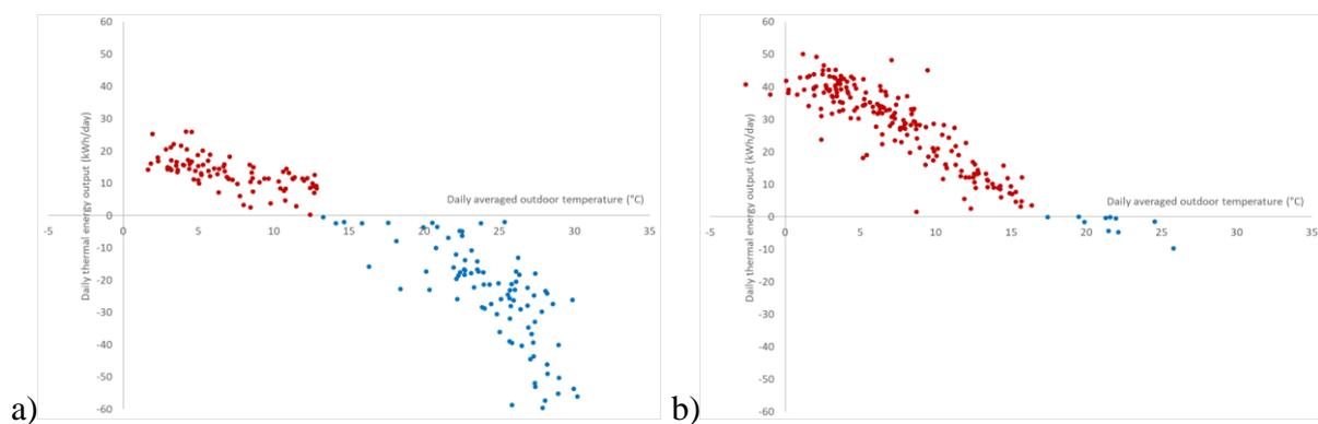
Figure 8: Energy signatures (daily thermal energy output as a function of daily averaged outdoor temperature) for heating in red and for cooling in blue for the house in Italy (a) and in Luxembourg (b).
