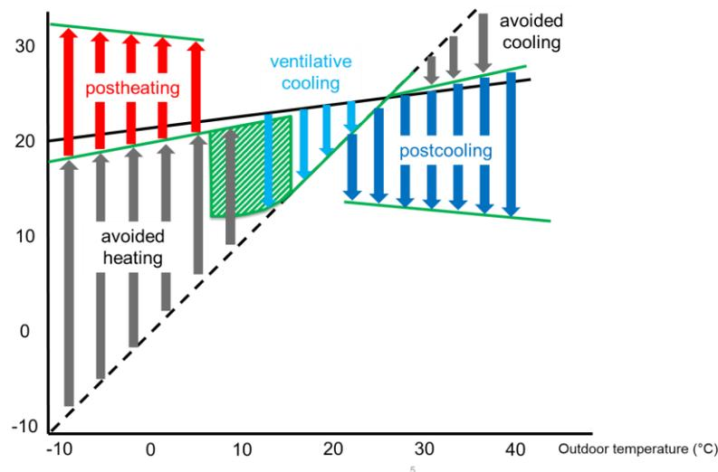
Figure 3: Schematic representation of the working principle. Black line: temperature of indoor air, green line: temperature of supply air (possibly after postconditioning)
